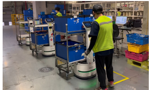
[Fig. 6] A typical example of an unloading station in a warehouse
