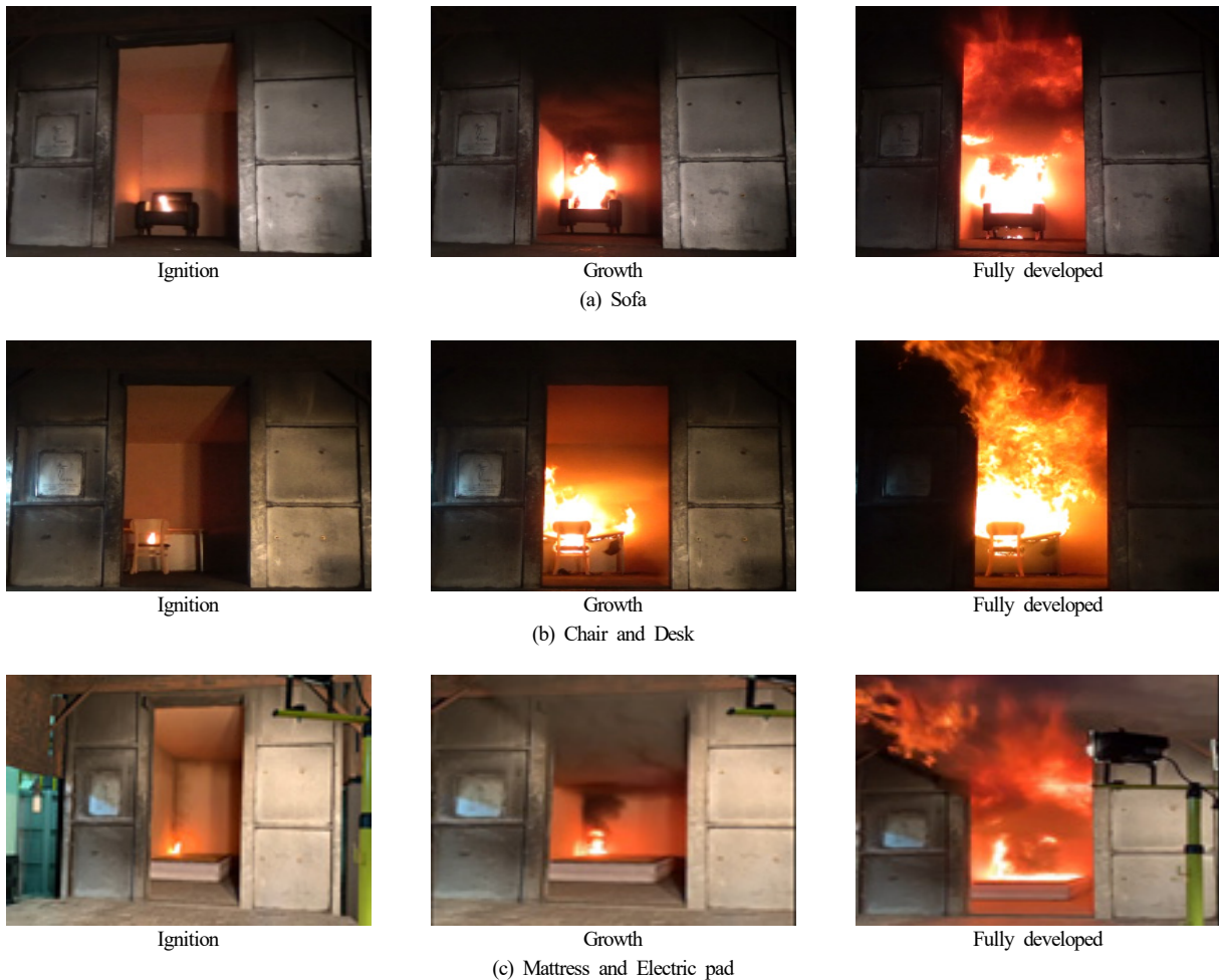
Fig. 4. Fire aspect according to fire growth stages for combustibles in test room.
