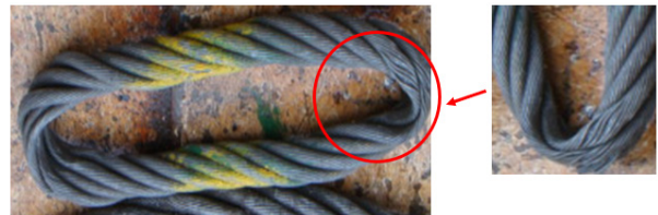
Fig. 4. Severe deformation case of grommet.
