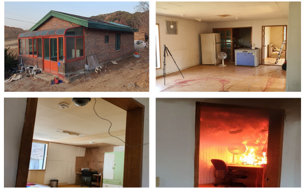
Fig. 4. Field photos of the real fire reproduction experiment.
