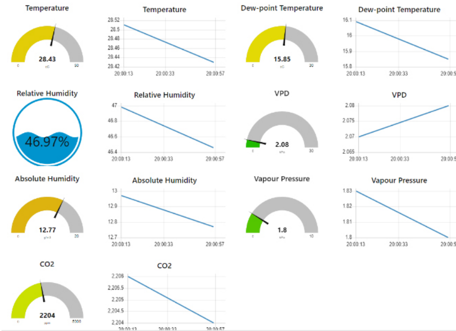
Fig. 4. Node-RED flows: (A) Master flow send command to a sensor node, (B) Master user interface display sensed data, (C) Slave flow receive data from a sensor node, and (D) Slave user interface display sensed data (Continued).
