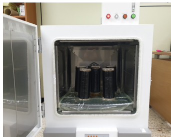
(e) Reinforced Concrete Curing (High Temperature)
