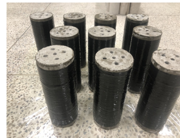
(f) Reinforced Concrete Curing (Normal Temperature)
