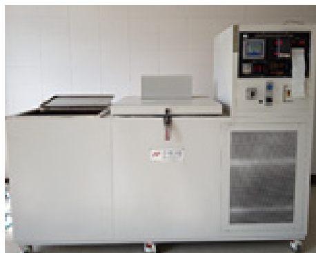
(a) Freezing and Thawing Test Machine
