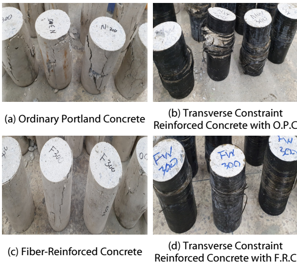
Fig. 9. Concrete Failure Form
