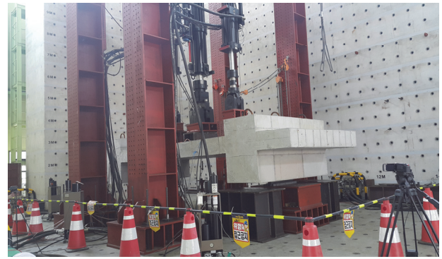
Fig. 8 Static load test for non-strengthened specimen
