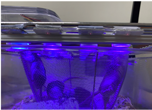
Fig. 1. LED-light therapy system for NC/Nga mice and application of phototherapy with 405 nm+850 nm light.
