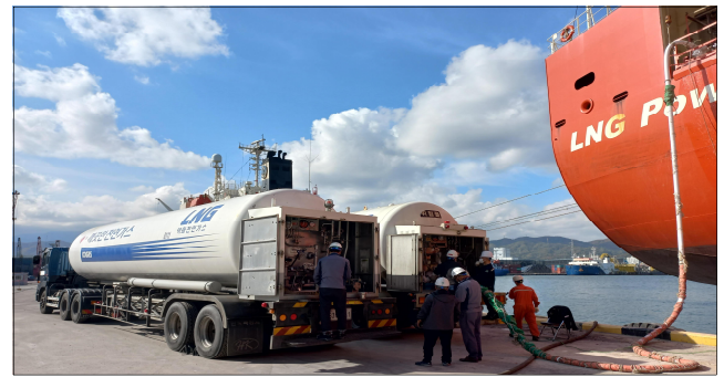
Fig. 4. Truck to ship LNG Bunkering. (Source: photo taken by the author)
