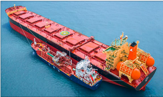
Fig. 5. Ship to ship LNG Bunkering (HL ECO). (Source: DNV, 2021)
