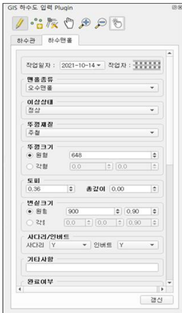
Fig. 5. Sewage manhole attribute input UI/UX design
