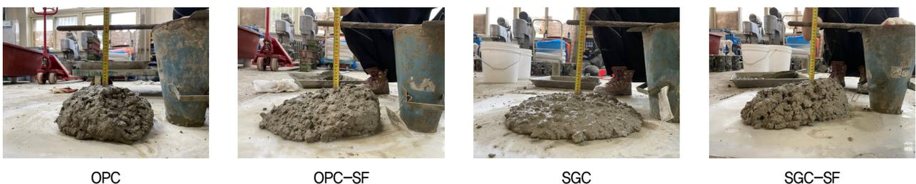
Fig. 5. Slump test for fresh RWM
