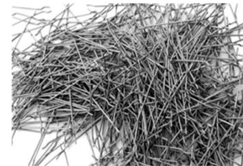
Fig. 1 Steel fiber(SF) used in this study
