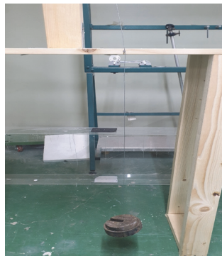
Fig. 7 View of applying cable tension
