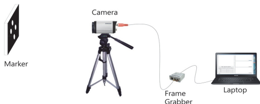
Fig. 5 Setup for visual displacement measurement
