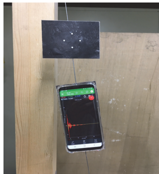
Fig. 8 Target for VDM and smartphone for acceleration measurement
