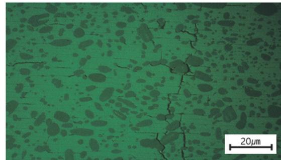
**Fig. 6.** Result of YBCO superconductor microstructure observation.
