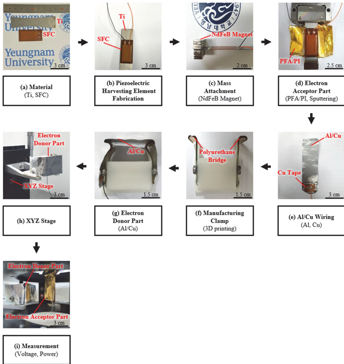
Fig. 4. Flow diagram of the overall experiment procedure; fabrication of piezoelectric harvester and triboelectric harvester, and characterization of hybrid energy harvester.
