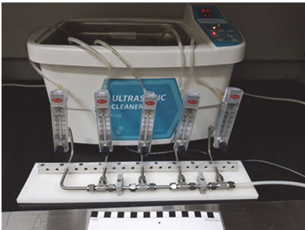
Fig. 2. Photography of the ultrasonic treatment with air-stripping facility.
