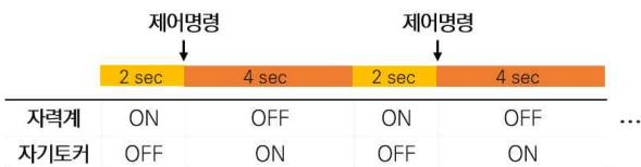
Fig. 5 Duty ratio of MTQ during initial detumbling
