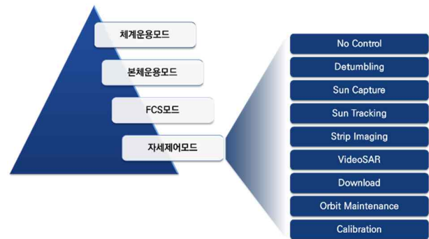
Fig. 4 Architecture of S-STEP operation mode
