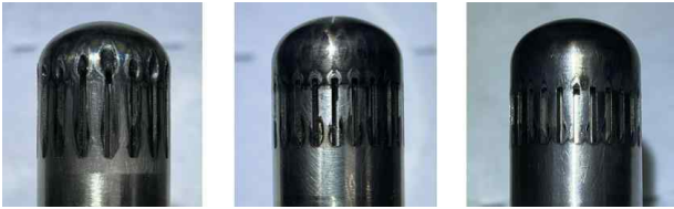
Fig. 11 P01, P02 and P03 Pintle tip after hot-firing tests
