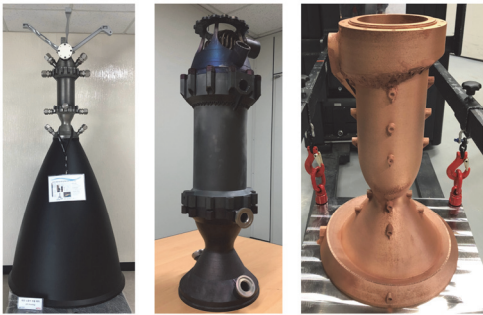
Fig. 10 3D printed combustion chambers. (left & center : Inconel 718, right : CuCrZr alloy).
