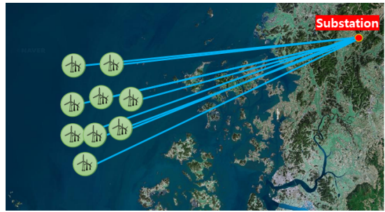
Fig. 2 Path diagram of the transmission system connecting each offshore wind farm to the substation with each line
