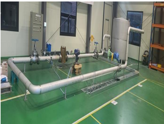
Fig. 4 Photograph of test equipment for measuring valve flow coefficient(Cv)
