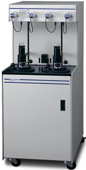
Fig. 2 Equipment for measuring the rate of porosity & diameter of pores (Autopore IV9500)
