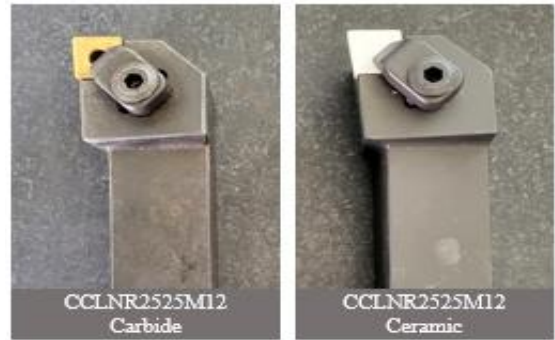
Fig. 2 Cutting tool assembly
