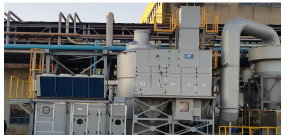
Fig. 1 Layout of cyclone type sludge drying system
