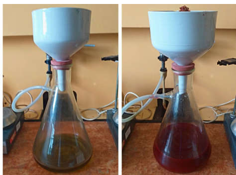
Fig. 4 H. perforatum herb extraction with chloroform (left) and methanol : acetone (2:1 w/w) (right)
