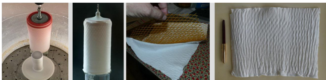
Fig. 1 Preparation of the PHB submicron fiber mat by the centrifugal spinning technology and a rotating fiber collector
