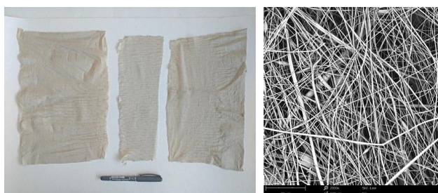
Fig. 7 PHB submicron fiber mat enriched by the H. perforatum extract prepared by the centrifugal spinning technology (left) and SEM image of microstructure of the fiber mat (right)
