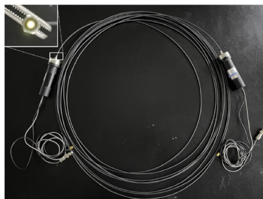
Fig. 1. Photograph of the end of the polished PSOF and an assembly after combining the 15 m length PSOF and two PMTs.
