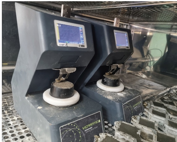
Fig. 1. Vicat test setup of cement paste (Vicamatic2)
