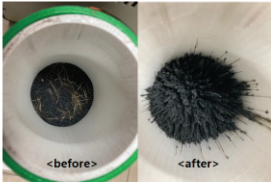
Fig. 12. Steel slag and fibers under magnetic field
