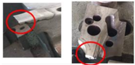
Fig. 3 Fracture phenomena of the tool during the cam-trimming process
