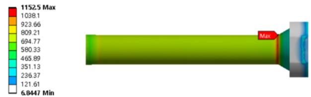
Fig. 6 Von-mises stress of stem
