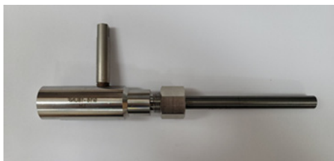
(a) Photo of waterjet nozzle mount
