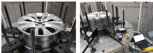
Fig. 1 Cornering Fatigue Test setting<sup>(4)</sup>
