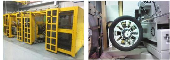
Fig. 2 Radial Fatigue Test setting
