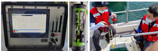
Fig. 7. Communication test between monitoring device and ultrasonic module.
