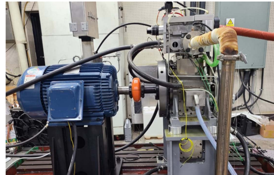
Fig. 1 Apparatus of floating liner engine
