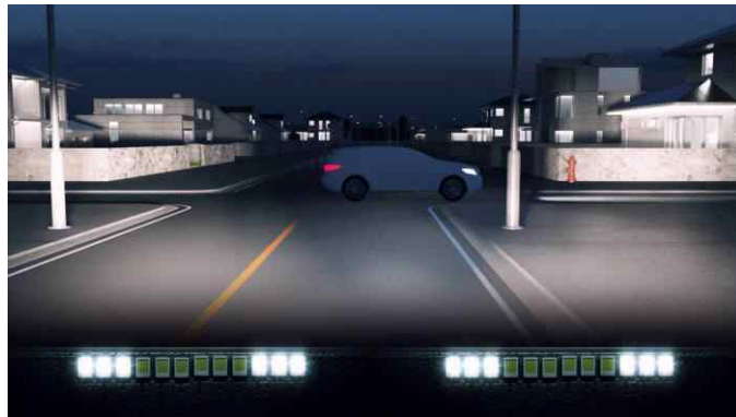
Figure 1. Intelligent LED headlamp operation simulation 1)
