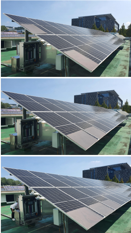
Fig. 2. Simulated partial shading using black sheets
