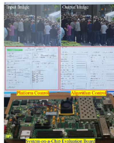
Fig. 4. Hardware verification using a system-on-a-chip evaluation board.
