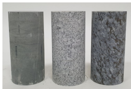
Fig. 1. Rock test specimens (shale, granite, granitic gneiss) used in this study
