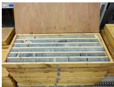
Fig. 1. Rock test specimens (shale, granite, granitic gneiss) used in this study
