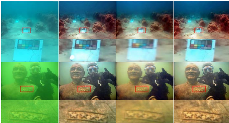
Fig. 10. Images recovered by different network architectures. From left to right: the original images, the images recovered without the attention mechanism, the SOS module, and the images recovered with the attention mechanism + SOS module.
