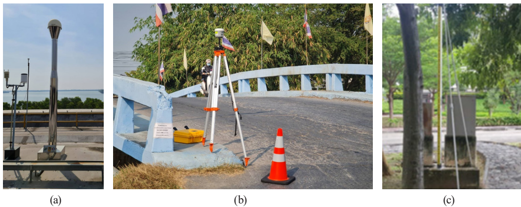
Fig. 2. The GNSS static surveying and precise spirit leveling: (a) THAI CORS and (b) GNSS observations using CHC i80 geodetic receiver, and (c) the barcode rod installed at an RTSD leveling benchmark
