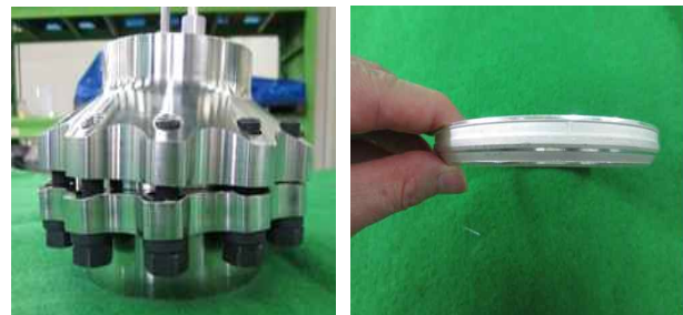
(a) Off Axis Assembly (b) Static Seal Fig. 3 Prototype of Spherical Flange
