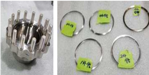
(a) Flange Tester (b) Static Seal Fig. 6 Visual Inspection after Test
