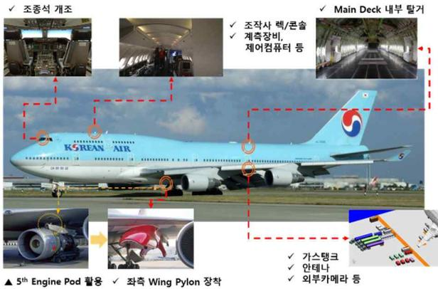
Fig. 3 Major Modification of Air Launcher Vehicle
