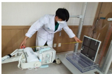
Fig. 6. Distortion image acquisition according to the detector angle
