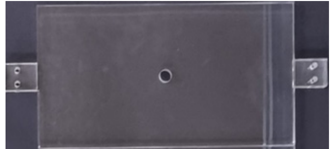
Fig. 6 Orifice on top of OWC chamber
