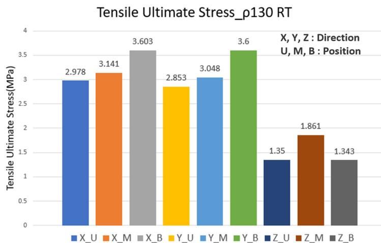
Fig. 11 Ultimate tensile strength of R-PUF by stacking position and coordinate direction for an R-PUF density of 130 kg/m<sup>3</sup> at room temperature
