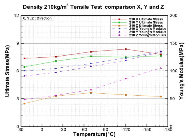
**Fig. 15** Density 210 kg/m<sup>3</sup> tensile test comparison X, Y and Z
