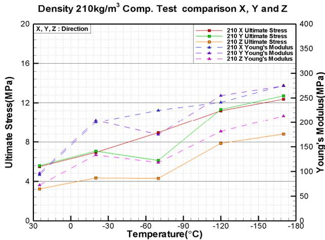
Fig. 20 Density 210kg/m<sup>3</sup> comp. test comparison X, Y and Z
