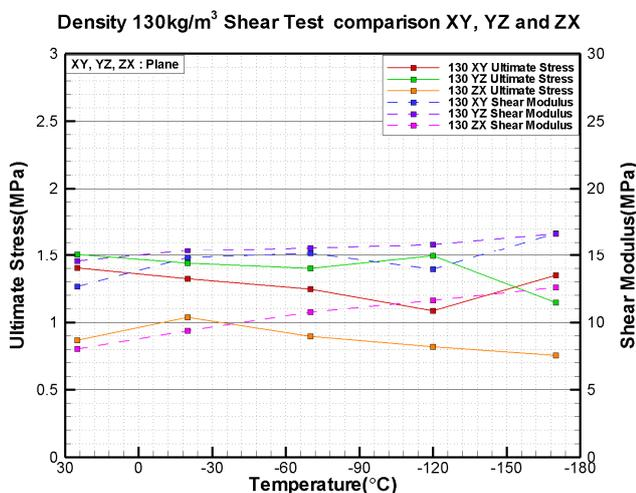
**Fig. 23** Density 130 kg/m<sup>3</sup> shear test comparison XY, YZ and ZX
