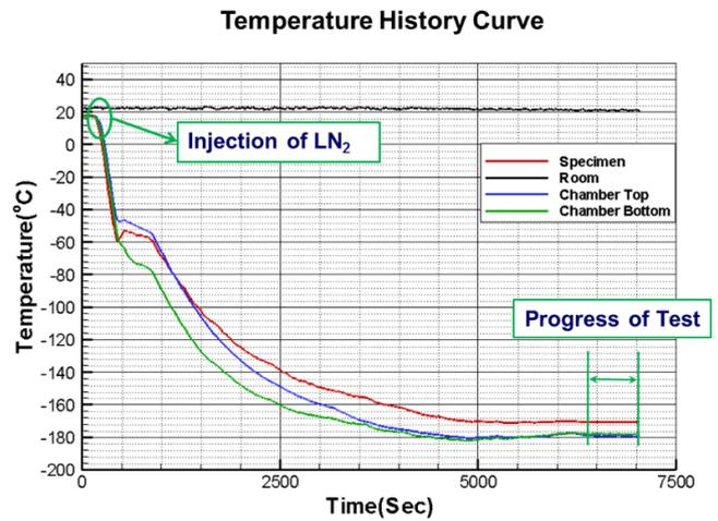
Fig. 6 Temperature history curves at various points during a typical test on R-PUF of this study
