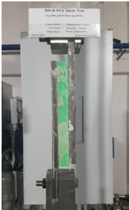
Fig. 10 Experimental setup for the shear test of R-PUF
