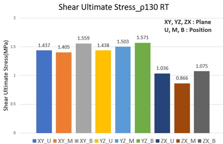
Fig. 21 Ultimate shear ultimate strength of R-PUF by stacking position and coordinate plane for an R-PUF density of 130 kg/m<sup>3</sup> at room temperature
