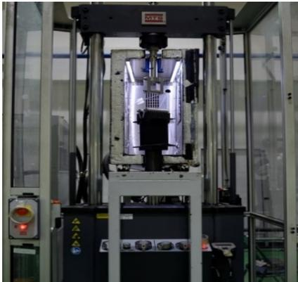
(a) 50 kN MTS universal testing machine used in the study
