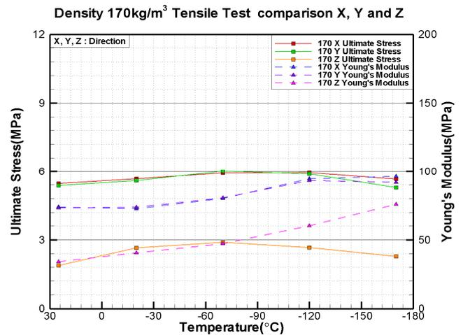
**Fig. 14** Density 170 kg/m<sup>3</sup> tensile test comparison X, Y and Z
