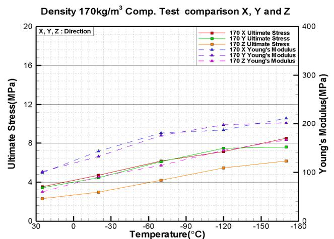
**Fig. 19** Density 170kg/m<sup>3</sup> comp. test comparison X, Y and Z
