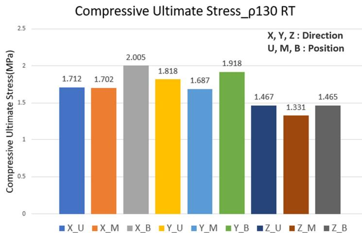
Fig. 16 Ultimate compressive strength of R-PUF by stacking position and coordinate direction for an R-PUF density of 130 kg/m<sup>3</sup> at room temperature
