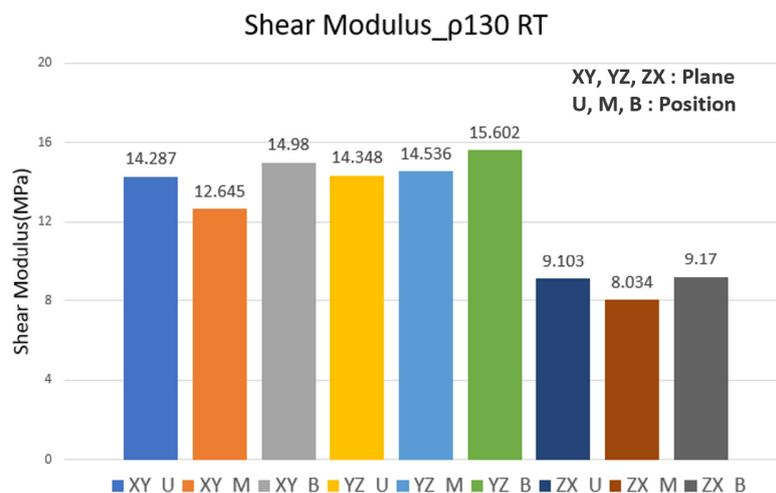
Fig. 22 Shear modulus of R-PUF by stacking position and coordinate plane for an R-PUF density of 130 kg/m<sup>3</sup> at room temperature
