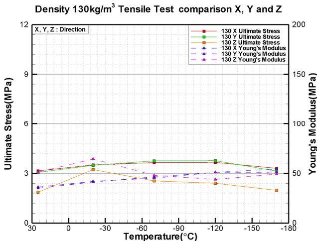
**Fig. 13** Density 130 kg/m<sup>3</sup> tensile test comparison X, Y and Z
