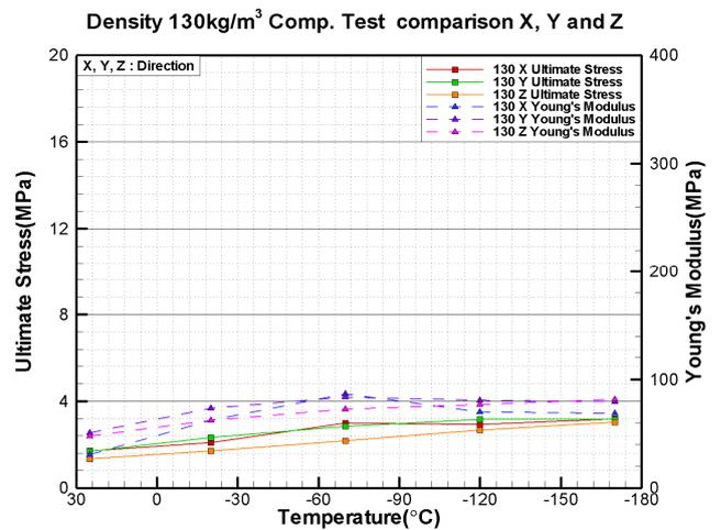
**Fig. 18** Density 130kg/m<sup>3</sup> comp. test comparison X, Y and Z
