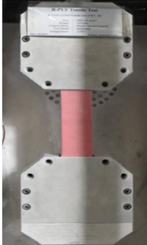
(a) XY planar view of the setup showing the R-PUF specimen
