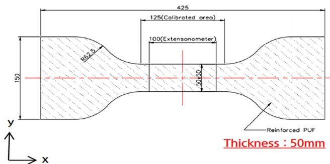
(a) Specimen dimensions on the XY plane
