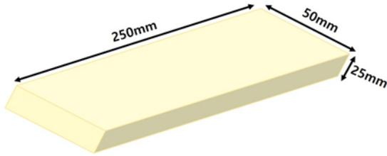
Fig. 4 R-PUF shear test specimen dimensions
