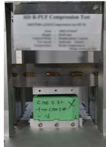
**Fig. 9** Experimental setup for the compression test of R-PUF
