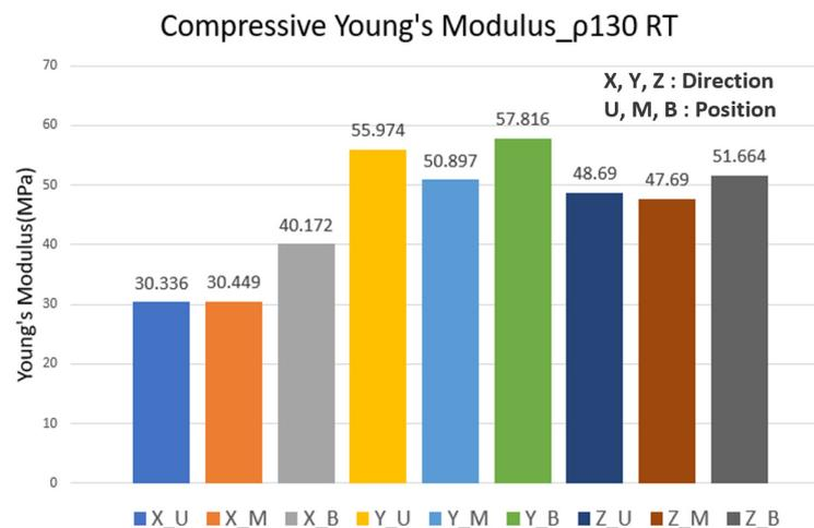
Fig. 17 Compressive Young's modulus of R-PUF by stacking position and coordinate direction for an R-PUF density of 130 kg/m<sup>3</sup> at room temperature
