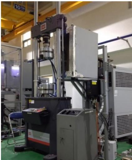
(b) 250 kN MTS universal testing machine used in the study
