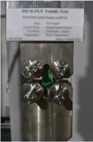
(b) Z-directional view of the setup showing the R-PUF specimen
