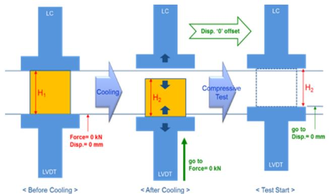
Fig. 7 Schematic R-PUF specimen shrinkage control during a cryogenic test of this study
