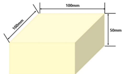
**Fig. 3** R-PUF compression test specimen dimensions
