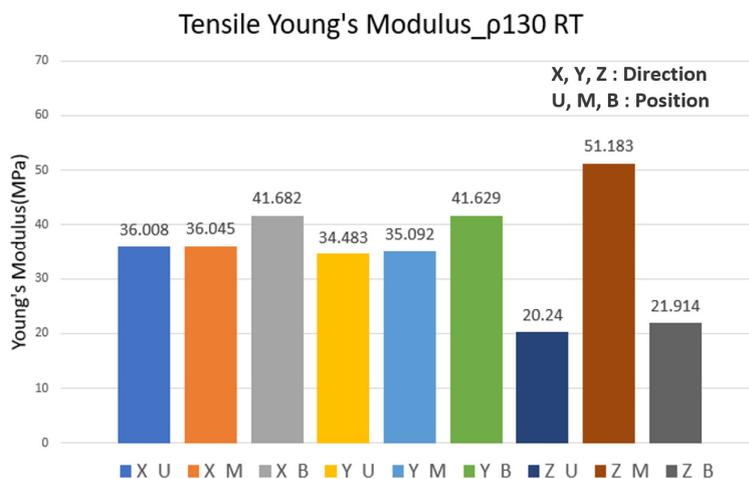
Fig. 12 Tensile Young's modulus of R-PUF by stacking position and coordinate direction for an R-PUF density of 130 kg/m<sup>3</sup> at room temperature
