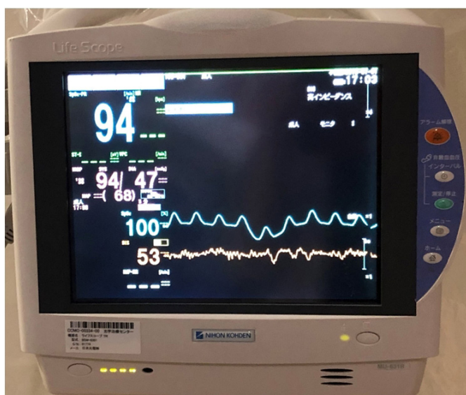
Fig. 1. The bispectral index monitor analyzes the brain waves and displays the calculated bispectral index value at the bottom of the screen.
