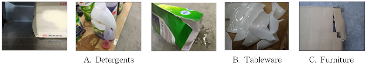
Fig. 4. Damages of the packaged products from the field-to-lab test.
