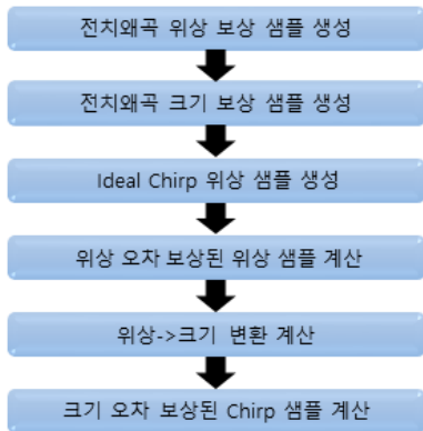
Fig. 3. Flow chart of chirp samples compensated for the magnitude and phase error
