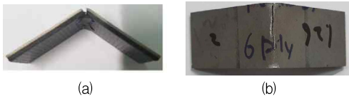
Fig. 4 Image of the tested specimen with reinforced compression action surface
