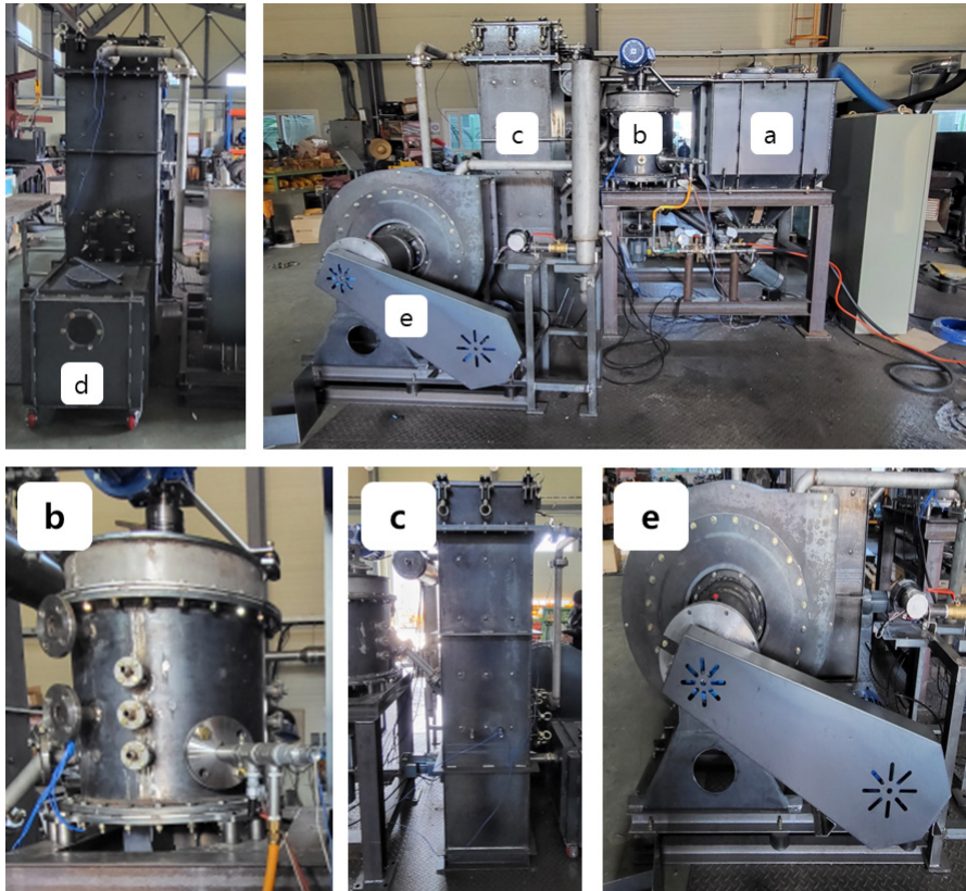
Figure 9. Gasification system of torrefied biomass using O 2 agent: (a) Torrefied biomass hopper (b) Gasifier (c) Gas cleaner (Ceramic filter) (d) Ash bucket (e) Hot gas blower.
