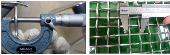
Fig. 16 Wave forming wire specimen dimension measurement
